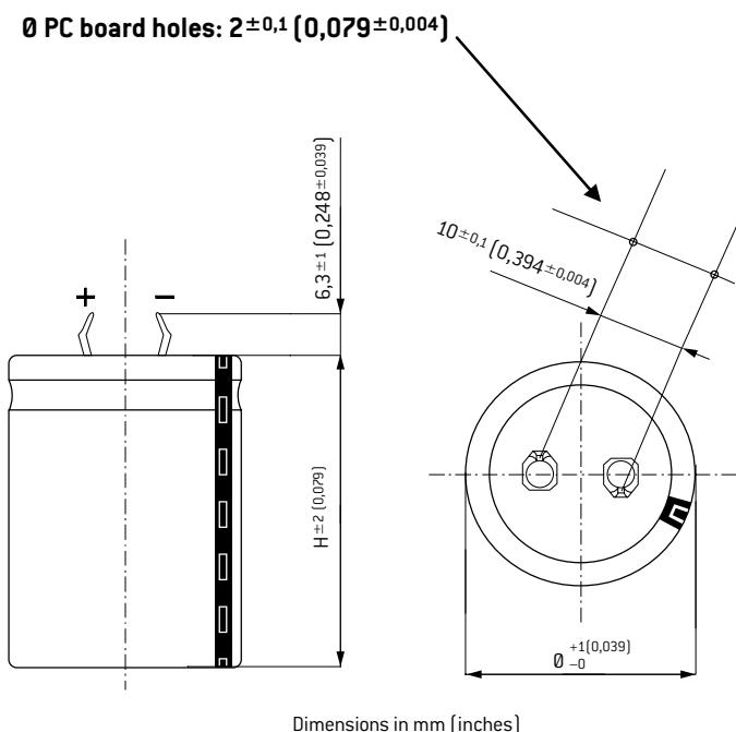
Standard pins can be replaced by 4,5 (0,177) max pins on request
