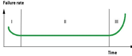
Failure rate is measured in FIT (failure in time =  $10^{-9} / \text{hour}$ ).
