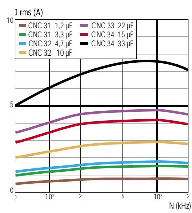
$U_{RC} = 25V$  DC (Typical curves for  $\Delta\theta = 20^\circ C$ ).
