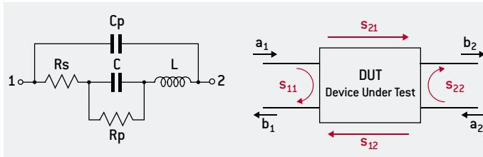
Figure 1: Equivalent Model
