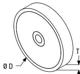
Discoidal capacitor with central lead
