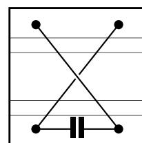
The total use of the the crossed four pole design allows operation at a higher operating frequency and reduces noise due to switching (lower self inductance) for a given capacitance value (see figures on the right).
