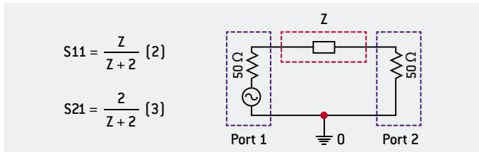
Figure 3: DUT Serial measurements
