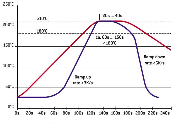
NB: the lines indicate the upper and lower limits of typical process (terminal temperature).
