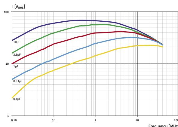
These typical curves are an example of admissible currents for one family of chip capacitors: 501R3740X chip series. For other curves and products or for further information, please contact us. Note: for the calculations, we have considered that the terminations are directly connected to an infinite heat sink. In other words, the thermal resistance of the circuit itself which depends of its type and design has not been taken into account. Moreover, the ambient temperature taken is 25°C.
