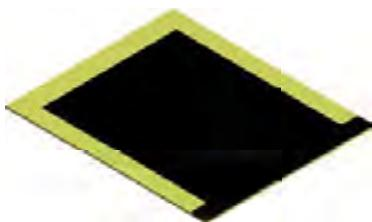
The electrode ink, made from a metal powder mixed with solvents, is printed onto the ceramic sheets using a screen printing process.
