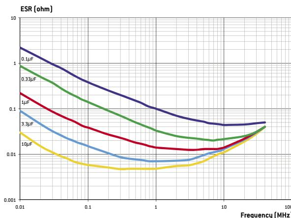
The ESR (Equivalent Serial Resistance) curves are given here for SMD (chips all case sizes) capacitors. Regarding the curves for the leaded capacitors, they are rather the same. Indeed, due to the resistivity of the raw material used and the wire diameters, the resistance of the wires is much lower than the ESR of the chips. So, in a first approach, their influence can be considered as negligible.
