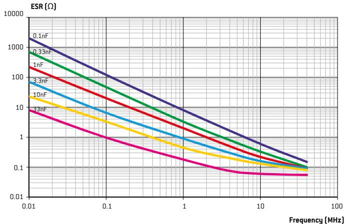
The ESR (Equivalent Serial Resistance) typical curves are given, here for SMD (chip) capacitors. Regarding the curves for the leaded capacitors, they are rather the same. Indeed, due to the resistivity of the raw material used and the wire diameters, the resistance of the wires is much lower than the ESR of the chips. So, in a first approach, their influence can be considered as negligible.
