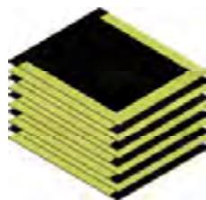
The sheets with electrode printed are stacked to create a multilayer structure.
