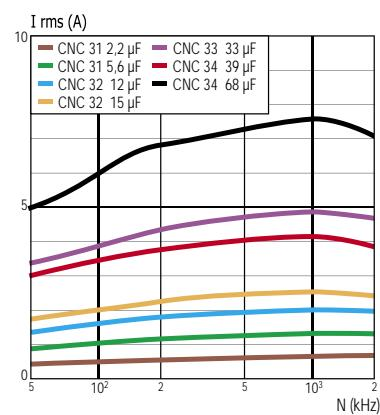
$U_{RC} = 16V$  DC (Typical curves for  $\Delta\theta = 20^\circ C$ ).
