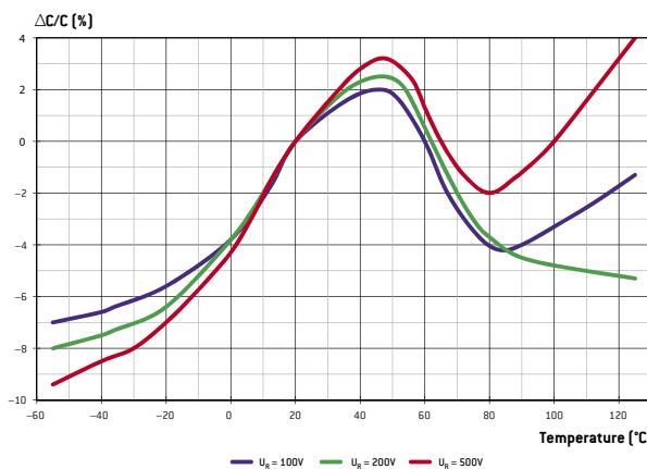
**T DIELECTRIC: TYPICAL TEMPERATURE COEFFICIENT WITHOUT VOLTAGE (for all sizes)**
