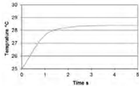
Example of the temperature evolution inside the capacitor
