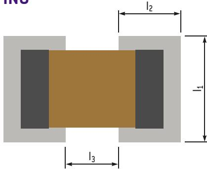
Large chips above size 2225 are not recommended to be mounted on epoxy board due to thermal expansion coefficient mismatch between ceramic capacitor and epoxy. Where larger sizes are required, it is recommended to use components with ribbon or other adapted leads so as to absorb thermo-mechanical strains.
