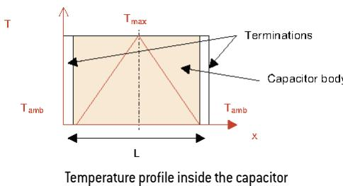
Temperature profile inside the capacitor
