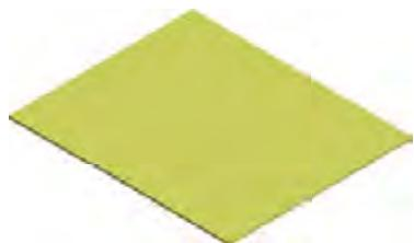
A slurry, a mix of ceramic powder, binder and solvents, is poured onto conveyor belt inside a drying oven, resulting in a dry ceramic sheet.
