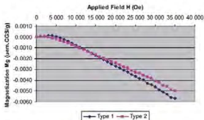
These two samples exhibit very similar diamagnetic behavior. The magnetic susceptibility  $X_g$  is in both cases around  $-1.6 \times 10^{-7} \text{ uem.CGS/g}$ .
