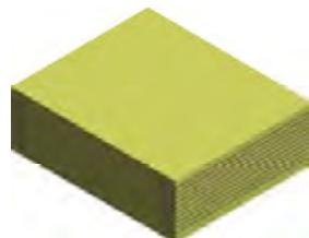
Pressure is applied to the stack to fuse all the separate layers, this created a monolithic structure.
