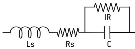
**The series inductance ( $L_s$ )** is due to the currents running through the electrodes. It can distort the operation of the capacitor at high frequency where the **impedance (Z)** is given as:
